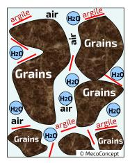
Soil is made up of different sizes of sand particles, clay, water and air. The sand particles, like the bones in the body, make up the skeleton of the brick, and the clay is the muscles. Durgin compression, water allows these elements to slide over each other to make a compact block, not too much and not too little is needed. To be strong, a compressed earth brick must have good bones and muscles!
