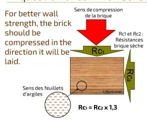
The resistance in the compaction directions is 30% higher than in the opposite direction.
