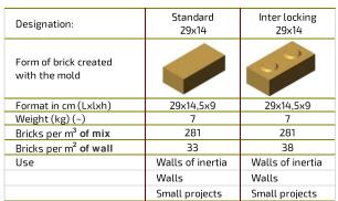
The MonoMeco produces bricks in the format 29x14,5x9, a set of interchangeable plates can make standard or interlocking bricks.
